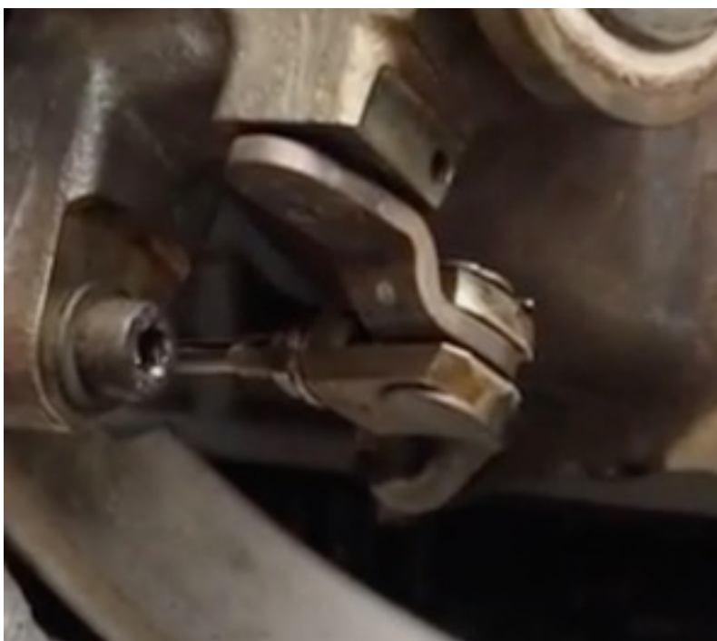
FIGURE 5 2015 VW IS38 TURBOCHARGER LINKAGE ROD END FORK
