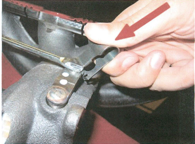
Figure 2. Fit the clip from the side.
