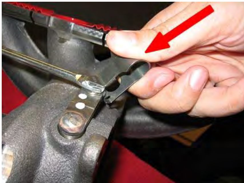
Figure 1. Fit the clip from the side.
