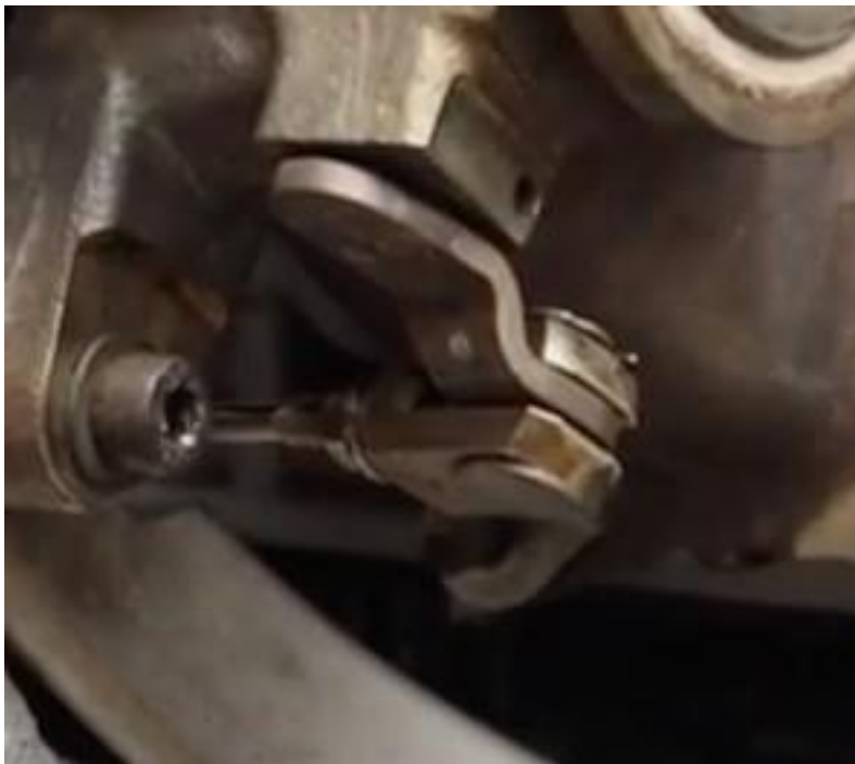
FIGURE 5 2015 VW IS38 TURBOCHARGER LINKAGE ROD END FORK
