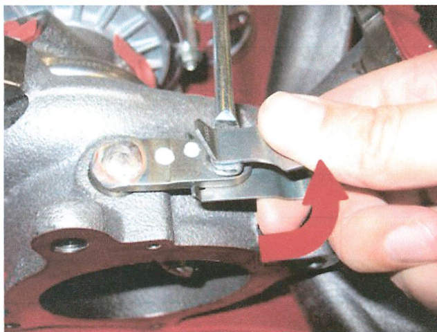
Figure 3. Turn the clip counter clockwise till the lugs slot in.
