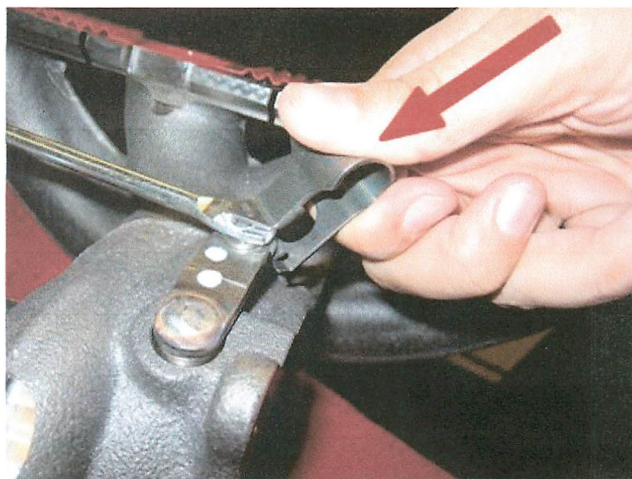
Figure 2. Fit the clip from the side.
