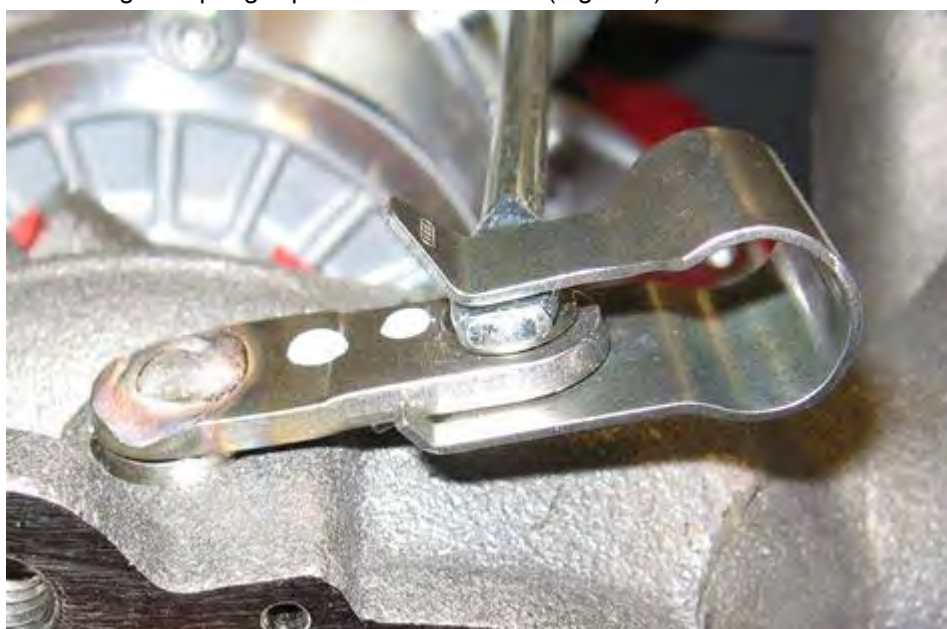
Figure 4. Correctly fitted clip.
