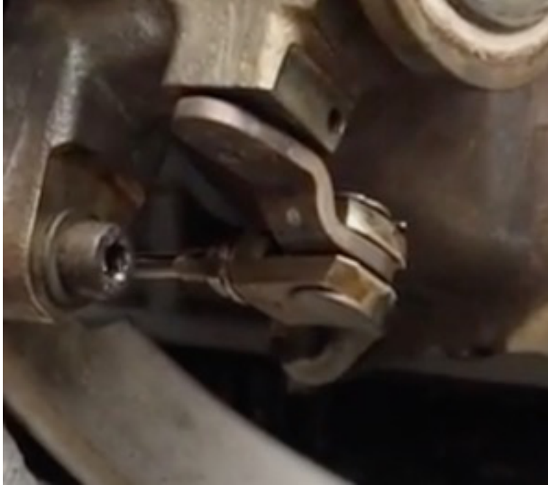
FIGURE 5 2015 VW IS38 TURBOCHARGER LINKAGE ROD END FORK
